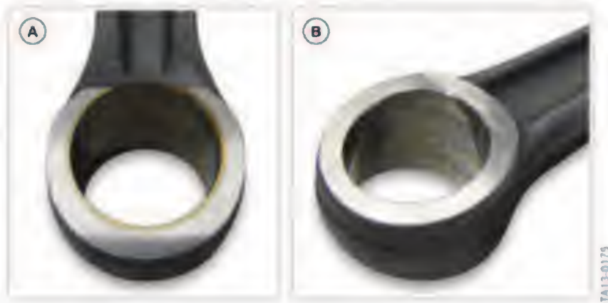
Connecting rod (B) without bushing in the N63TU engine
